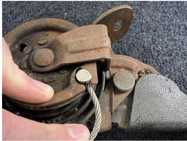
Figure 8: Uninstall the factory front cable from the park brake handle assembly
