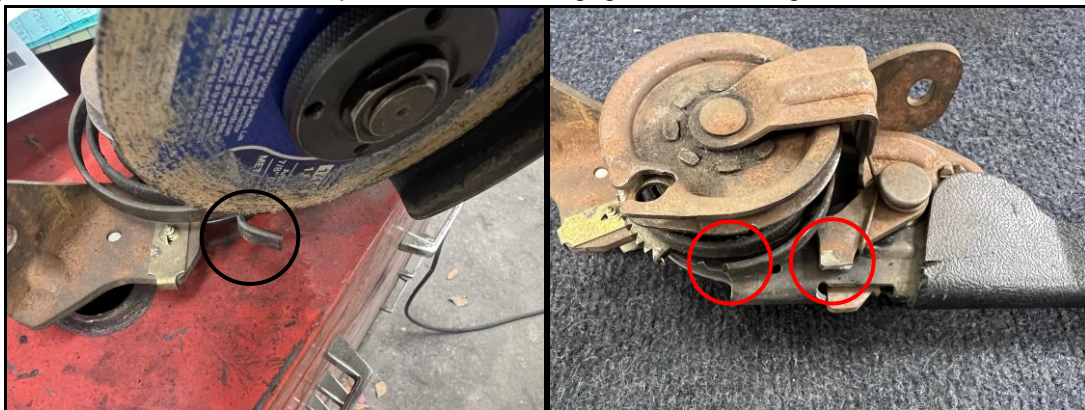
Figure 9: Grind small tab from self-adj. spring Figure 10: Grind top tab to let handle sit parallel to floor
