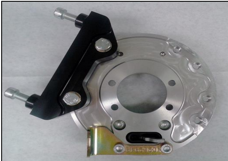
Figure 3: Park brake assembly correct orientation when installed (Inboard View)
