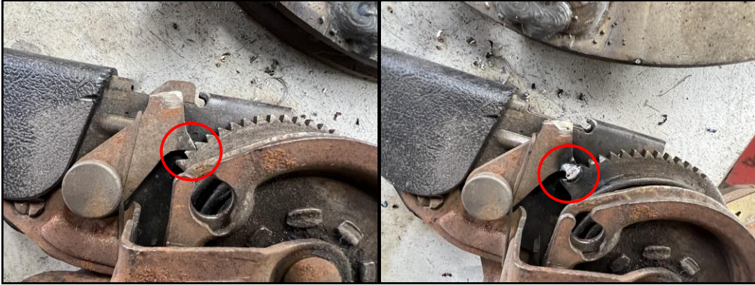
Figure 11: Weld location, second-to-last tooth Figure 12: Weld the paw to the handle
