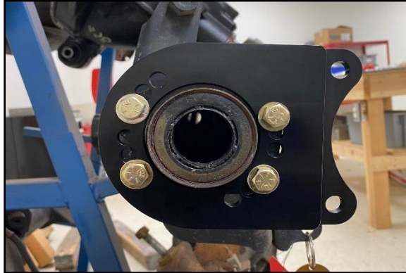
Figure 1: Base bracket installation (driver's side shown – bracket is engraved 6710135)
