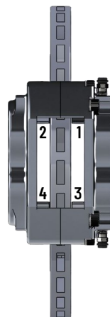
SS4+ SYSTEMS: MEASUREMENT LOCATIONS (SYSTEM COMPONENTS NOT INCLUDED FOR PHOTO CLARITY)
