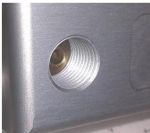
Figure 4: Insert correctly installed
