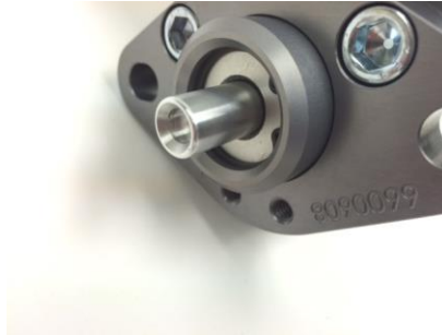
Figure 2: Master cylinder bullet (short pushrod booster)
