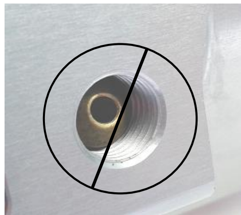
Figure 5: Insert incorrectly installed
