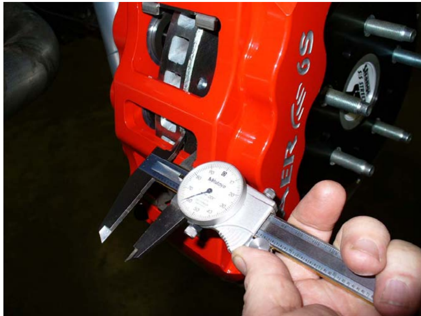
Measure from rotor to caliper body
