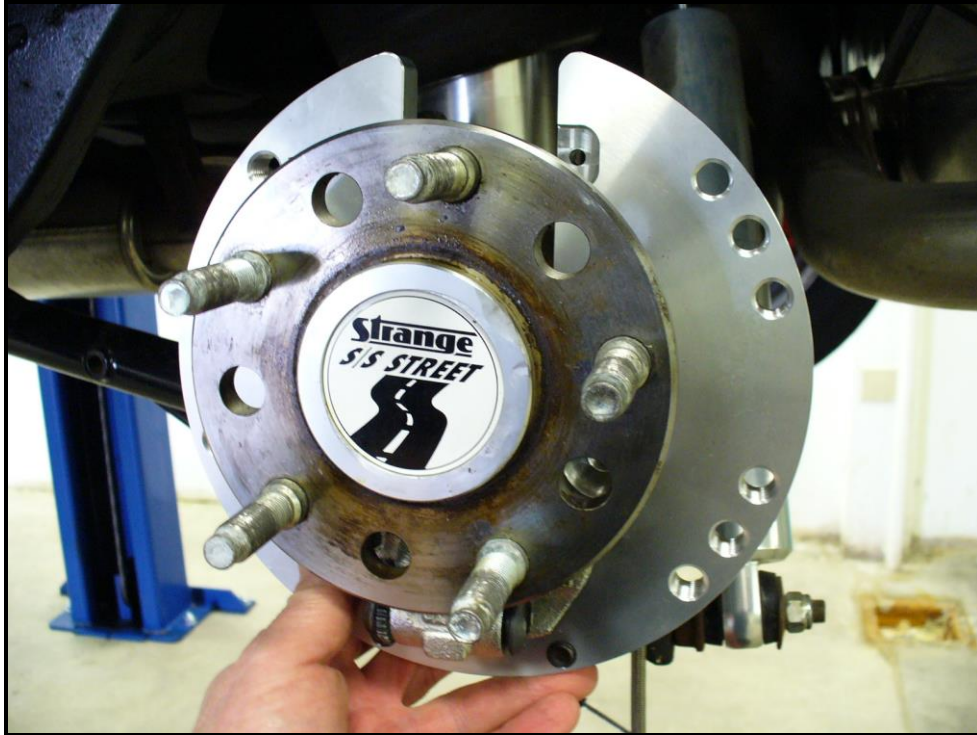
Various mounting positions for the caliper
