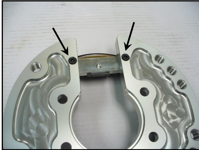
Shoe retainer allen screws
