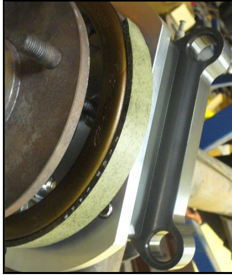
Figure 3: Park brake assembly correctly installed
