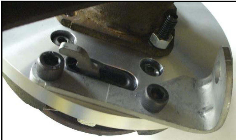
Figure 4: Park assembly installed on driver's side (Actuator is shown at the bottom)
