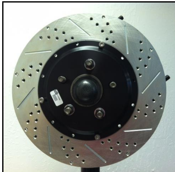
Figure 4: Left rotor temporarily secured with lug nuts and washers
