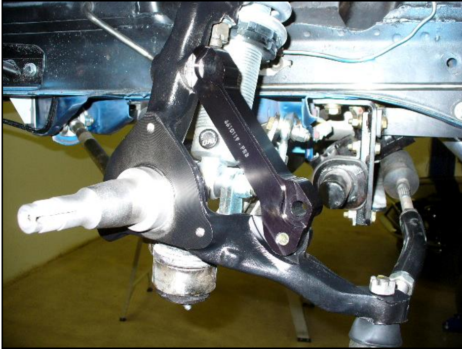
Figure 2: Left bracket installed, caliper to rear of spindle pin
