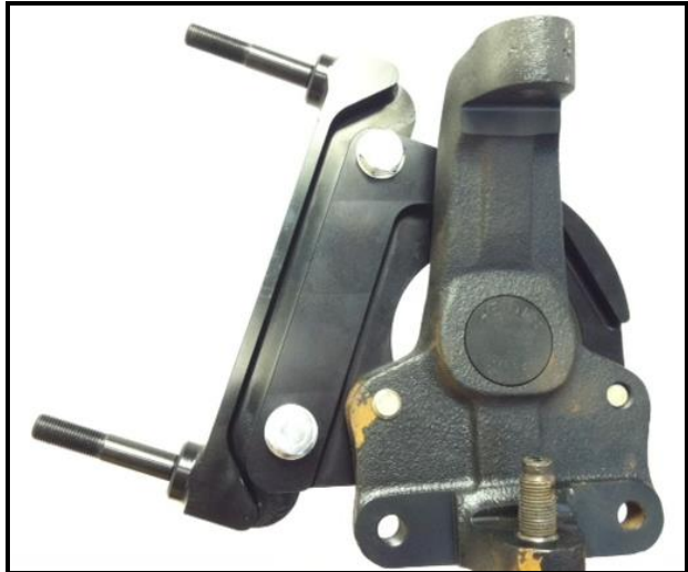
Figure 11: Rear view- bracket installation
