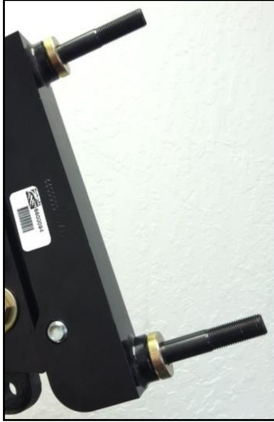
Figure 12: Spacers installed over radial mount studs
