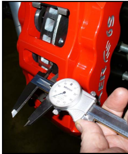
Figure 13: Measuring distance from rotor to caliper body
