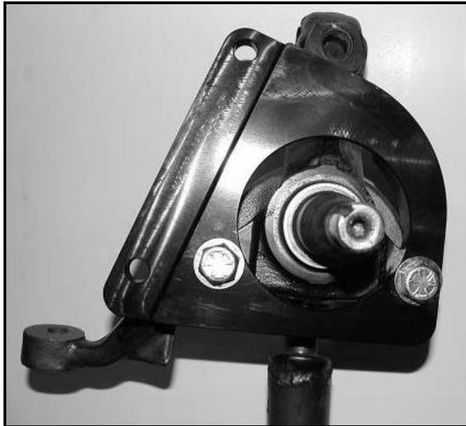
Figure 4: Rear Steer spindle shown with base bracket
