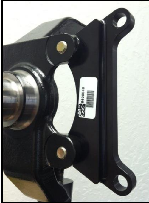
Figure 3: Bracket installed onto spindle
