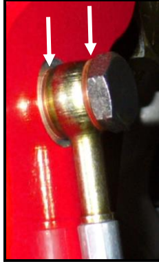
Figure 7: Installation of hose and washers
