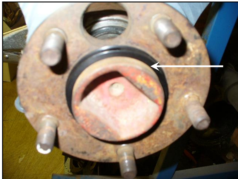
Figure 3: Black centering ring installed over rotor register
