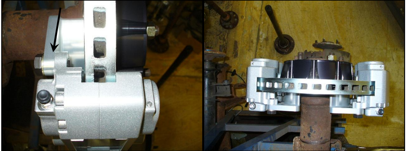
Figure 4: Arrow indicates shim placement.
