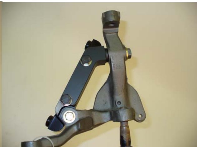
Inboard view of radial mount bracket
