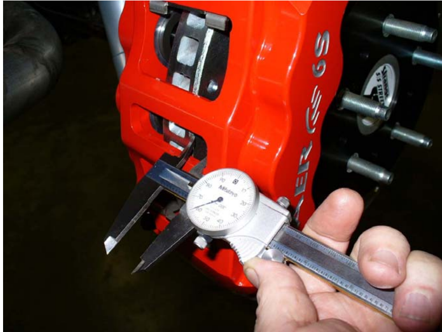
Measuring distance from rotor to caliper body
