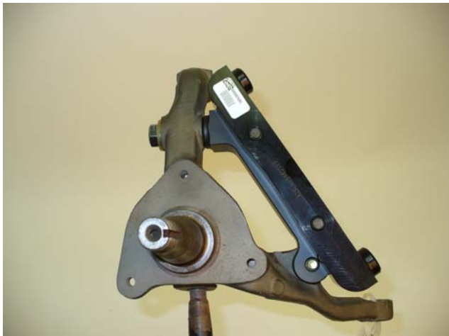
Outboard view of radial mount bracket
