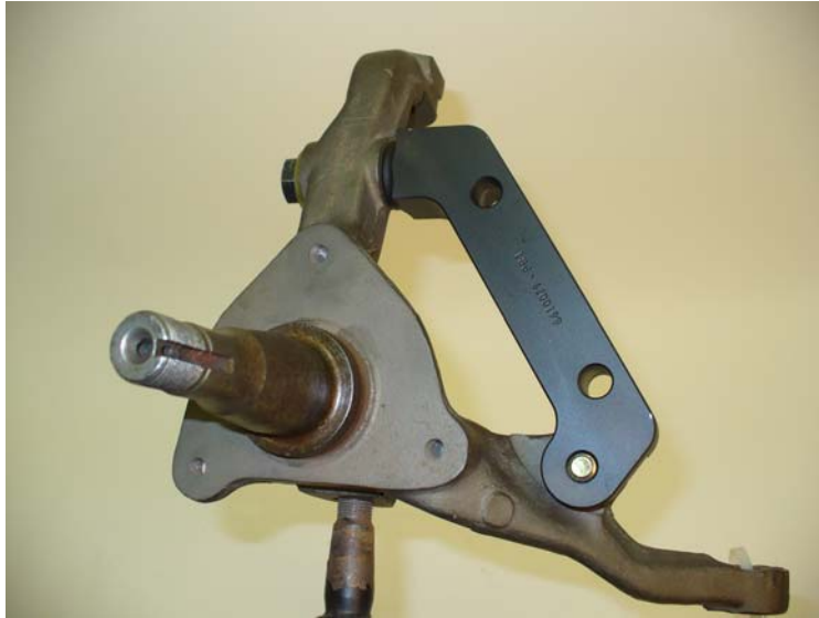
Left spindle with intermediate bracket installed
