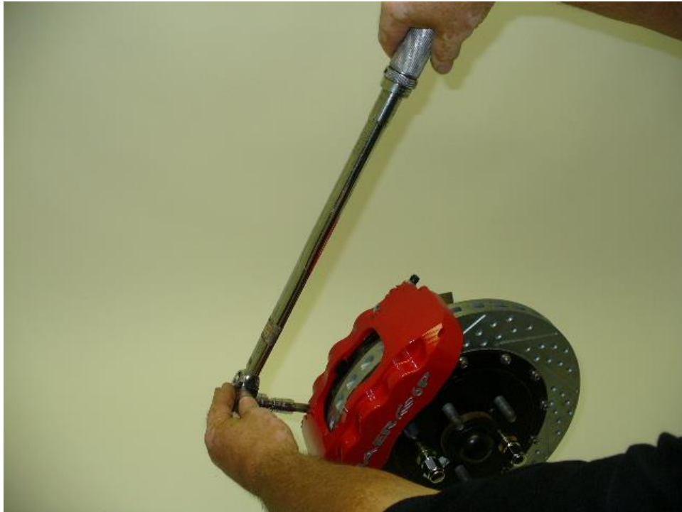
Torque caliper bolts to 85 ft-lbs.
