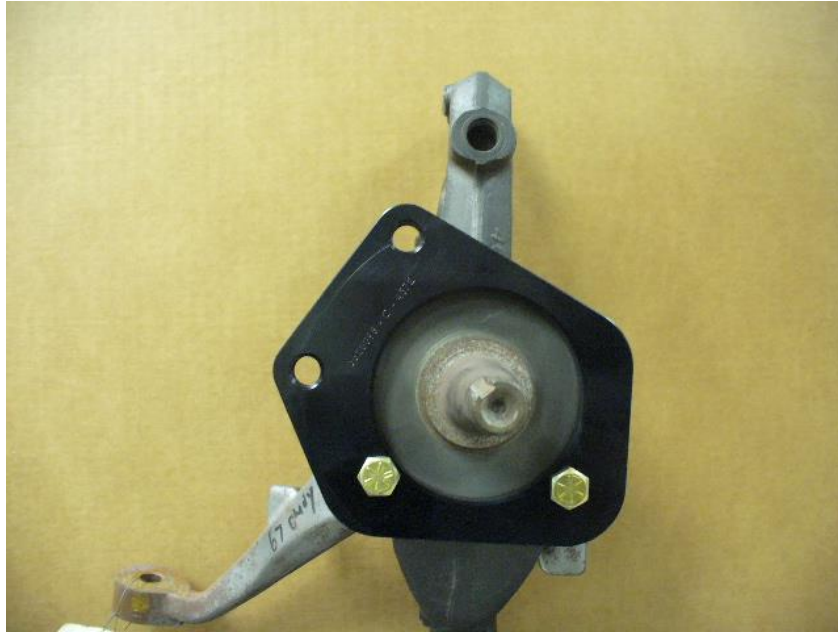
Spindle bracket mounting for Rear Steer applications Do not use washers under these bolt heads as they will interfere with the Baer hub.
