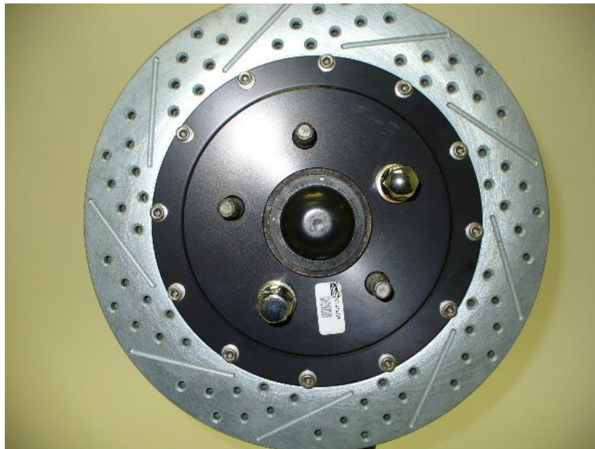
Secure rotor with 2 lug nuts and washers.
