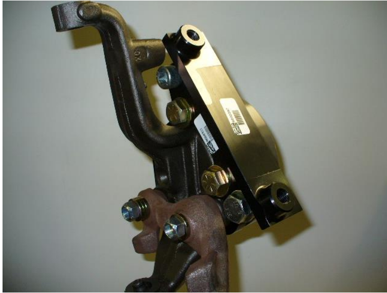
Radial mount bracket installed.
