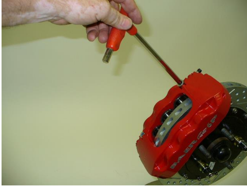
Install the caliper to measure clearance.
