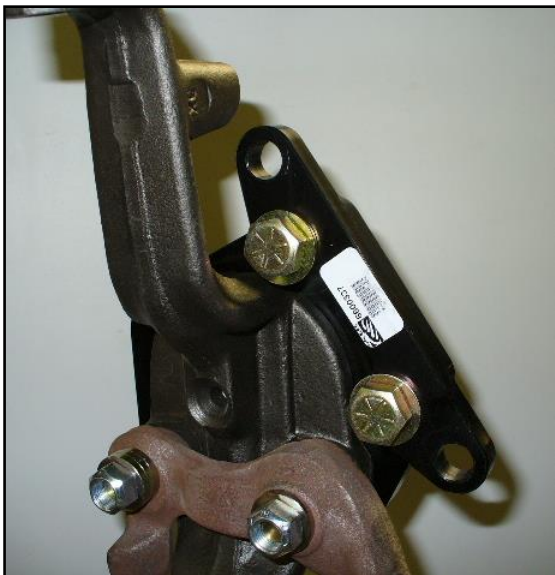
Intermediate bracket placement.
