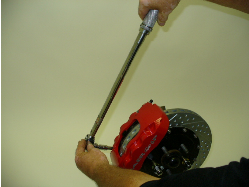
Torque allen bolts to 85 ft-lbs.
