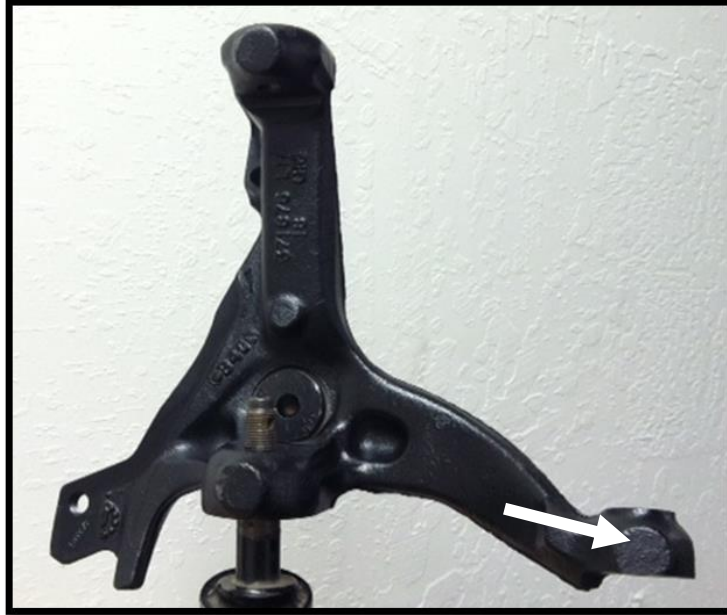
Figure 3: Strike tie rod end boss here with large hammer
