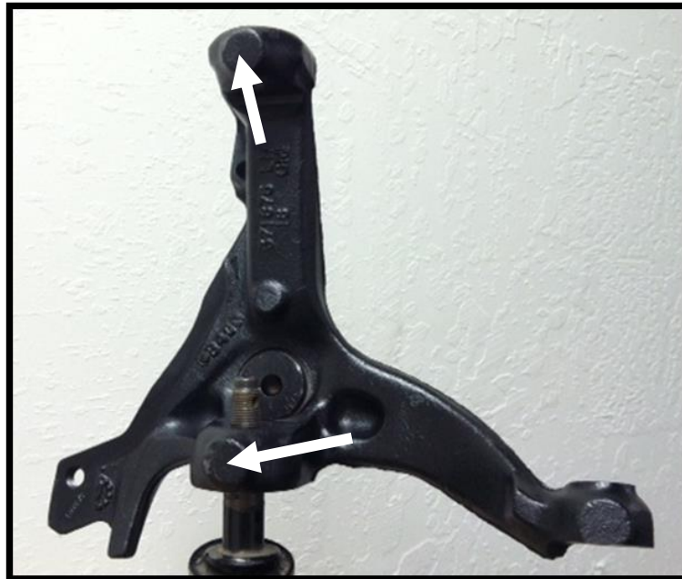
Figure 4: Strike at the indicated locations to dislodge ball joints
