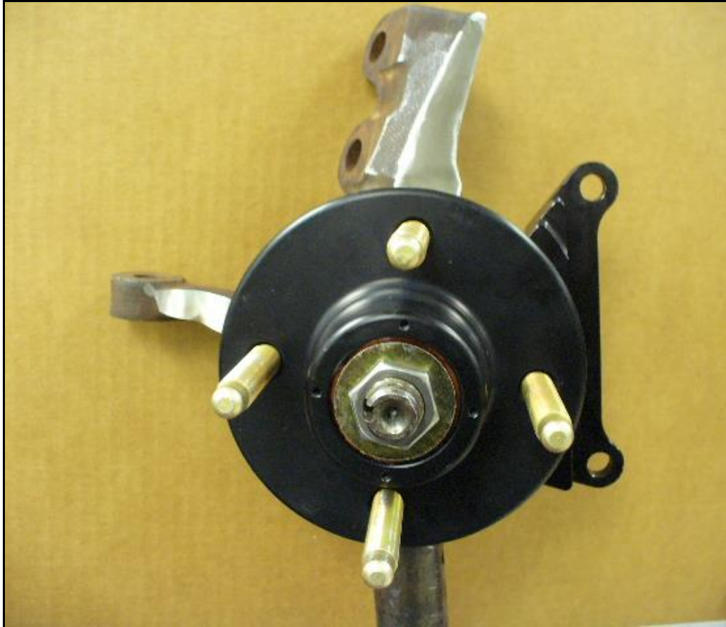
Hub installed with both brackets in place.
