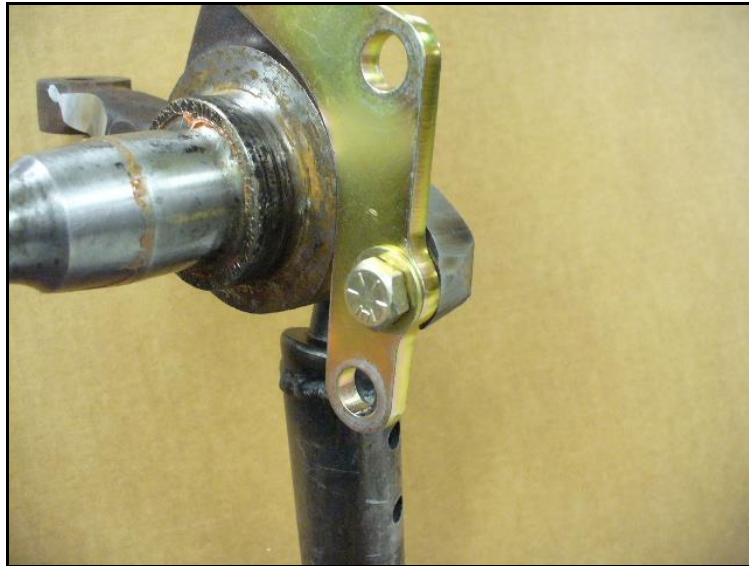
Intermediate bracket installed (short bolt in this location)
