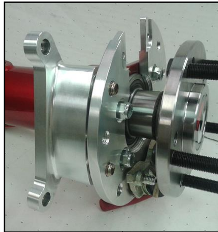
Figure 3: Intermediate bracket installed
