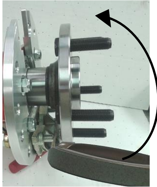
Figure 4: Install shoe into actuator from the bottom, rotate over hub
