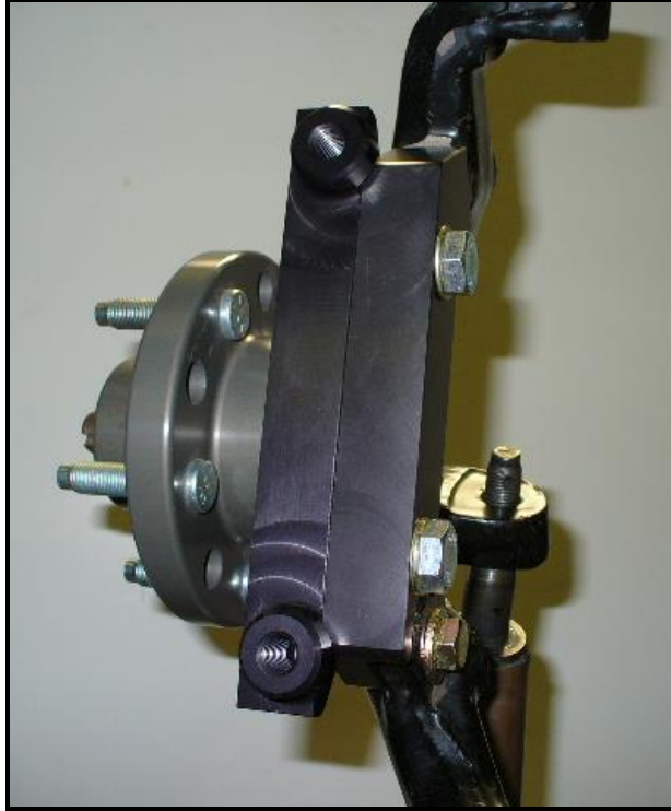
Figure 3: Intermediate bracket installed
