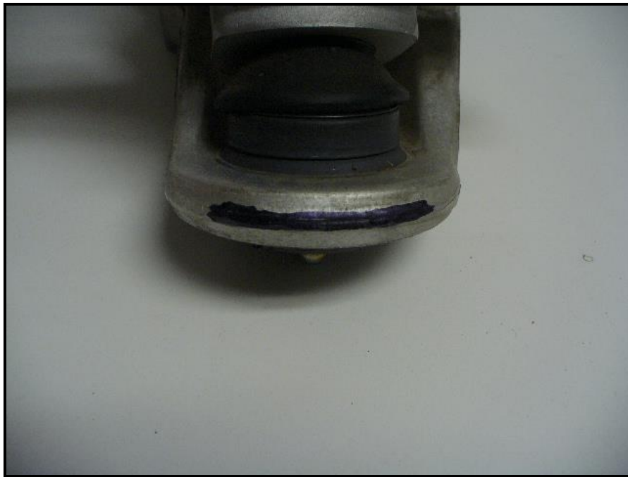
Figure 6: Area which may require trimming for rotor clearance
