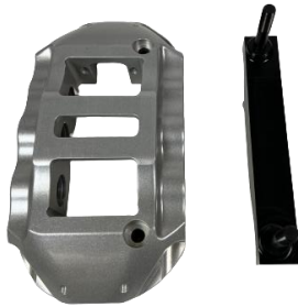
Figure 7: Align the mounting holes of the Baer 6S / XTR brake caliper with the ARP studs
