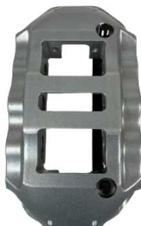
Figure 8. Slide the Baer 6S / XTR brake caliper over the ARP studs
