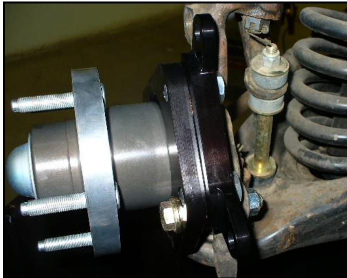
Figure 5: Intermediate bracket installed. Part number engraved on bracket faces outward
