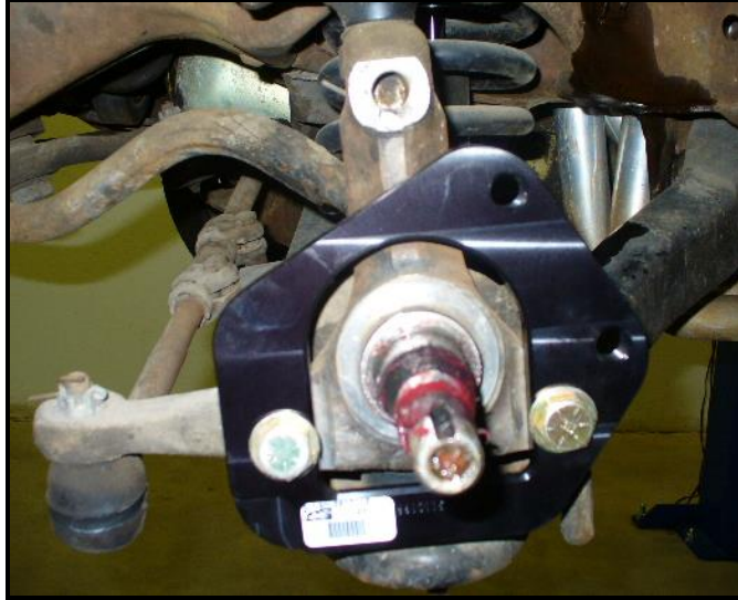
Figure 2: Left bracket installed, caliper to rear of spindle pin
