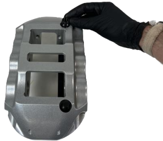
Figure 11: Temporarily secure the brake caliper to the intermediate bracket with the supplied ARP 12-point nuts
