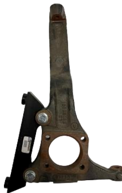
Figure 7: Intermediate bracket installation (wheel hub not installed in photo, ARP studs not installed in photo)
