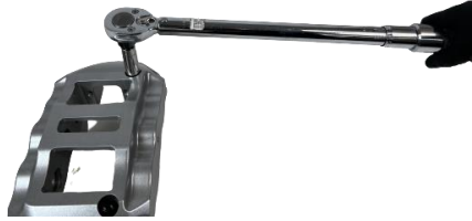
Figure 12: Torque the ARP 12-point nuts to 85 ft-lbs.
