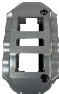
Figure 9. Slide the Baer 6S / XTR brake caliper over the ARP studs
