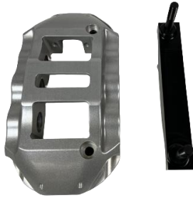
Figure 8: Align the mounting holes of the Baer 6S / XTR brake caliper with the ARP studs
