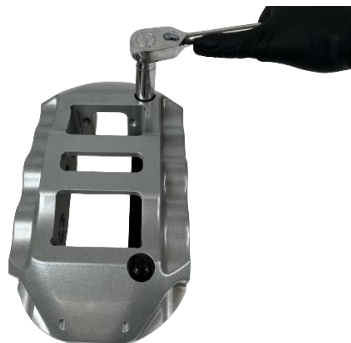
Figure 11: Following the shimming procedure, tighten the provided ARP 12-point nuts
