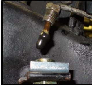
Figure 1: Hardline capped with supplied vinyl cap
